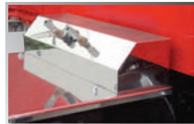
Air Line Boxes and Frame Panels
